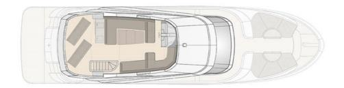
The MCY 70 open flybridge (bottom) vs. the Skylounge model (above) has the stairs moved from the aft deck to inside the salon. The outdoor grill is also moved inside as a refreshment center. And finally, the helm has been moved from the port side to a midship position.
