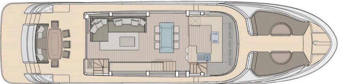
Cubierta principal con cocina en proa | Main deck with galley located forward
